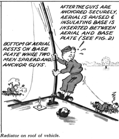
Erecting Vertical Radiator on roof of vehicle.
