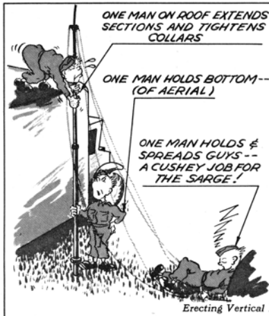
Erecting Vertical Radiator on roof of vehicle.
